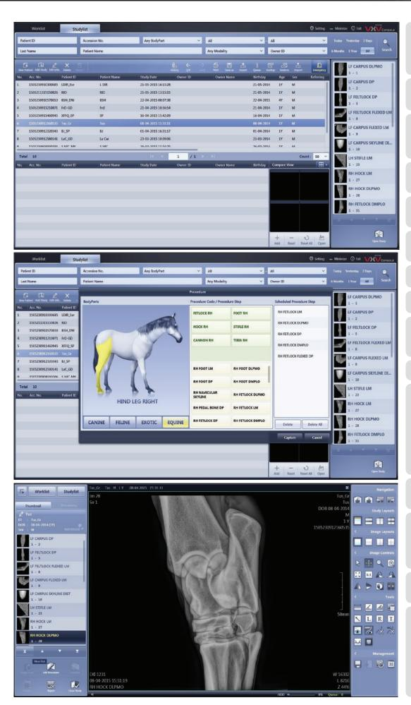
A fully integrated solution. Functions as an image acquisition console, image reviewer and database storage
